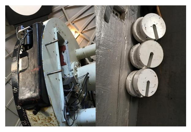
Two arc shaped weights were tied to one end of the ballast. The tape value is then 45-3/4":
